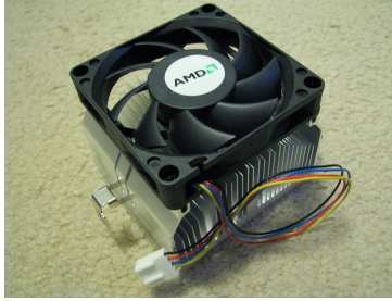
Example: AMD CPU heatsink
