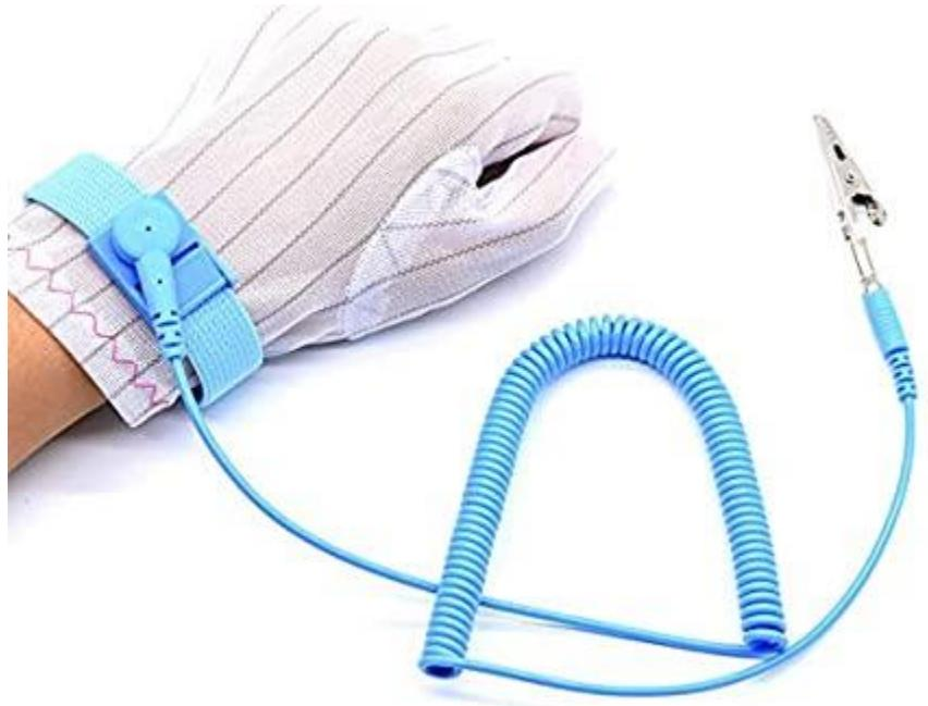
Severe PC assembly should use anti-static wrist strap and other anti-static equipment. Touching a grounded enclosure or other grounded metal objects is sufficient to eliminate the risk of electrostatic discharge and damage to PC components. However, it is best to wear anti-static equipment to be cautious. The main purpose of these tools is to prevent workers from discharging static electricity and prevent damage to PC components.
