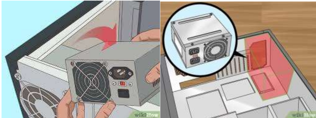
Figure 62: Installing power supply
