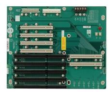
The function of the PCI slot is to allow you expand computer capabilities. PCI stands for Peripheral Component Interconnect. This is a computer slot that allows you to insert expansion cards into your computer. These can come in the form of sound cards, RAID cards, SSDs, graphics cards, NIC cards, Co-processors, and several other functional computer parts. So it enables you to expand the capabilities of the PC by adding what you do not have.
