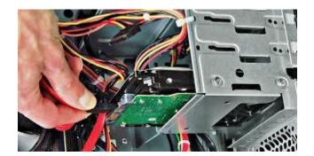
**STEP 3:** Connect the SATA cable and the IDE to the CD ROM Drive and Hard Disk and also connect the power supply cables to the drivers in the case. Then form the cables accordingly so that it saves space in the casing so that the heat gets released.
