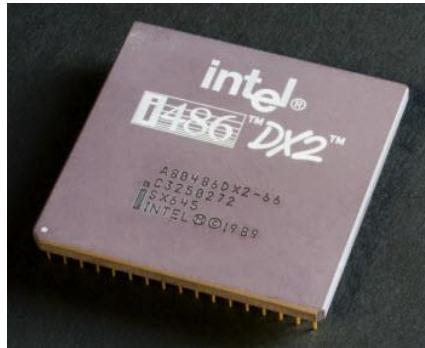
A photograph of an Intel i486 DX2 processor. The chip is rectangular with a gold-plated metal base. The text 'intel', 'i486', 'DX2', and 'INTEL' are printed on the chip. There is also some smaller text and a date '1989'. | <i>CPU/Processor</i> | A piece of hardware that carries out the instructions of a computer program.                                                                          |
