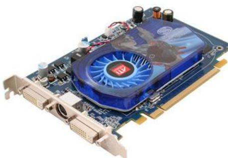
A photograph of a graphic card (GPU). It is a blue printed circuit board with a large blue heatsink and fan in the center. There are several ports on the side, including DVI and VGA.                                      | <i>Graphic card</i>  | A piece of computer hardware that produces the image you see on a monitor.                                                                            |
