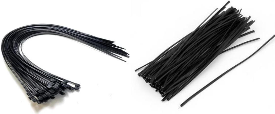
The zip ties and twist ties are used to tie any cables in a place. Zip ties, normally made of nylon are strong and single-use. Twist ties are secure and easy to remove but it have potential to scratch the cable because it made of metal wire. The importance of this tool is we can manage the cables well and keep better airflow in PC case. The cables also will look neat in term of cable management.
