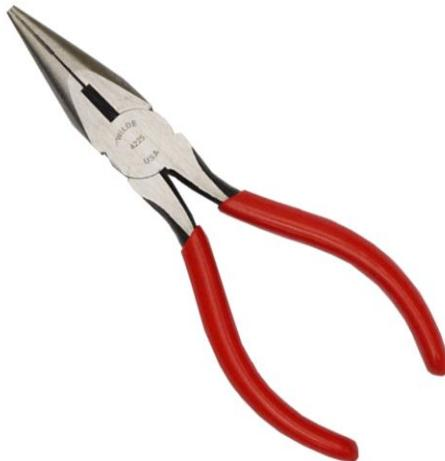
The pliers are used when we want to remove or insert small components. The importance of pliers is we can use it in various situations. As example, we can use pliers to pick up small screws that fall in the case, remove or insert jumper on hard drive and cut the excess zip ties.
