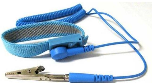
The anti-static wraps is used to eliminate electro-static discharge (ESD).The importance of this tool is to prevent us from damaging component with ESD. Sometimes, we cannot feel ESD so anti-static wraps can be used as precaution before anything happens.
