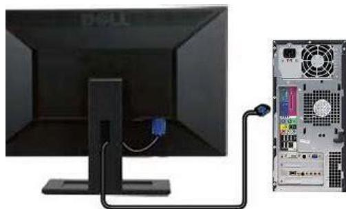
Finally connect the CPU with monitor by plugging into display ports.
