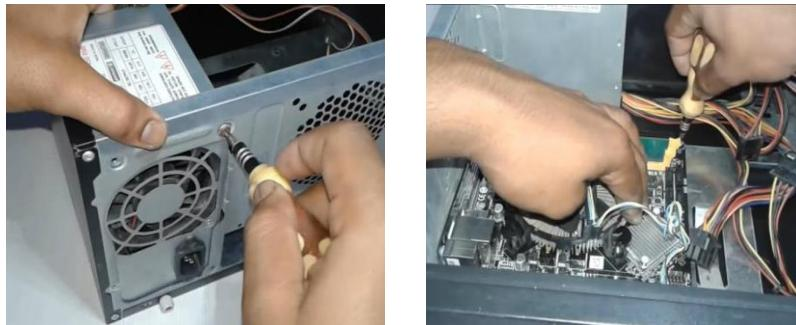
Install the power supply and the motherboard into the chassis plate and tightened the screws at every parts of the computer case respectively.
