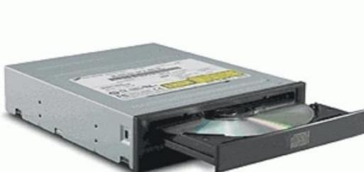
CD ROM is defined as compact disc read only memory. Thus, its function is to read data store in computer such as graphics, audio and text. The data in the disc only can read and cannot be written. Examples of model of CD ROM are Intel CD ROM and Asus CD ROM.
