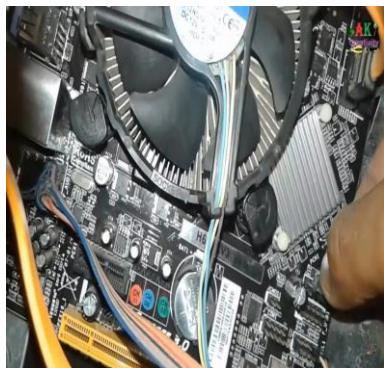
Connect the switch wire and USB of the chassis plate to the motherboard.
