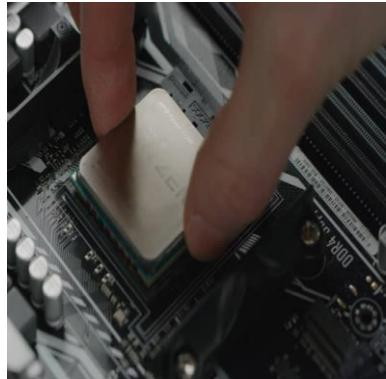
Insert the CPU on the motherboard and apply some thermal paste.
