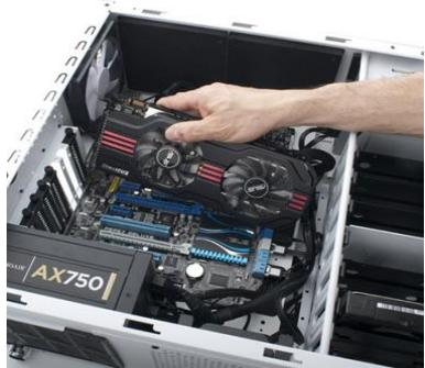
Install graphic card at the slot PCI-E and screw at the graphic card holder so that it is tidy and will not unplug easily.
