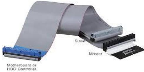
IDE cables are used to connect hard drives and optical drives to each other and to the motherboard in parallel connection. The two most common types of IDE ribbon cables are the 34-pin cable used for floppy drives and the 40-pin cable for hard drives and optical drives.
