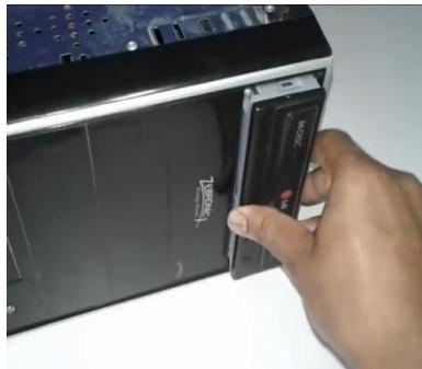
Install the CD ROM Drive into the chassis plate.
