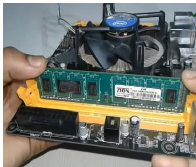
Install the pieces of RAM into the slot of the RAM.
