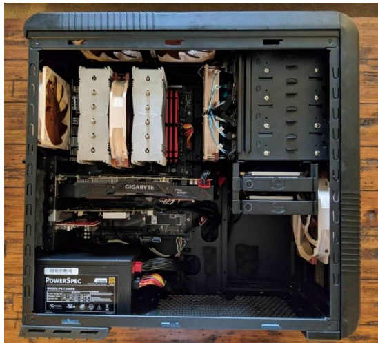
Example of a well cable management PC
