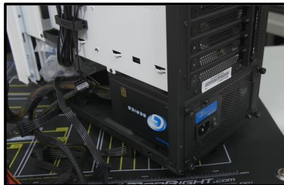
Picture 3.16 Install power supply
