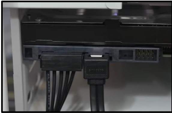
Picture 3.23 Connect SATA cables from motherboard
