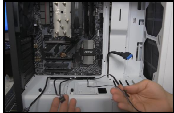
Picture 3.18 Route panel connectors through cutouts in CPU cutouts
