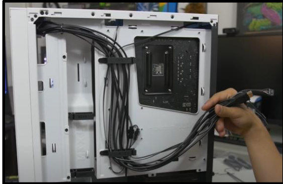
Picture 3.17 Front panel connectors
