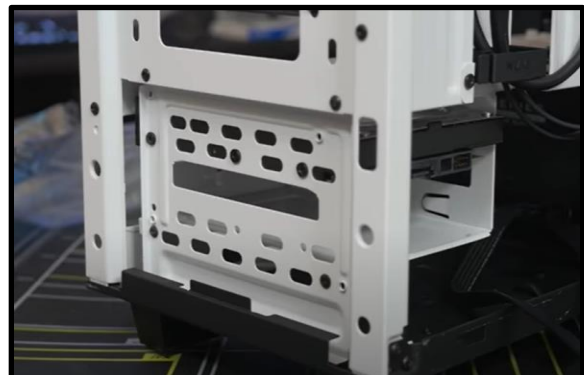
Picture 3.22 Install hard disk
