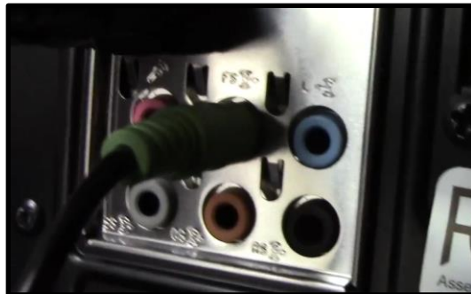
Picture 3.31 Plug in speakers into 2.5mm sockets
