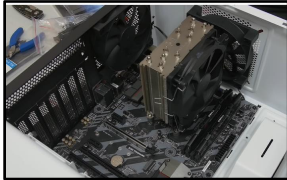
Picture 3.14 Install motherboard
