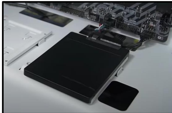
Picture 3.25 Install SSDs
