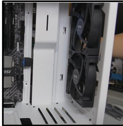
Picture 3.20 Install fans (optional)
