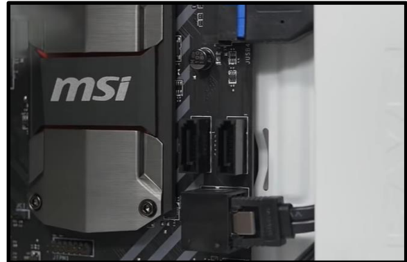
Picture 3.24 SATA port at motherboard and power supply
