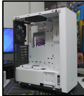
Picture 3.10 Remove side panel
