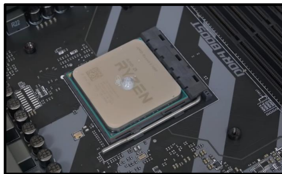
Picture 3.5 Apply a thermal paste
