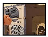
Place the side cover back on and secure the side panels with case screws.
