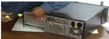
Figure 30. Secure the side panels with case screws. From Asas Pemasangan Sistem Komputer (ESS207) ( https://www.youtube.com/watch?v=ctK58A71DTs , accessed 11/12/2020)
