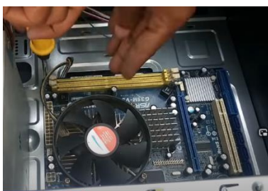
Figure 15. Tighten the screw of motherboard. From How to Make or Assemble Desktop CPU Step by Step At Home | How to Build a Computer with used Parts . ( https://www.youtube.com/watch?v=m - G9Cacx2U , accessed 11/12/2020)
