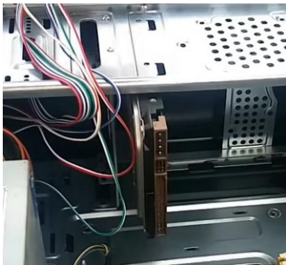
Figure 19. Mount hard disk into case. From How to Make or Assemble Desktop CPU Step by Step At Home | How to Build a Computer with used Parts . ( https://www.youtube.com/watch?v=m - G9Cacx2U , accessed 11/12/2020)
