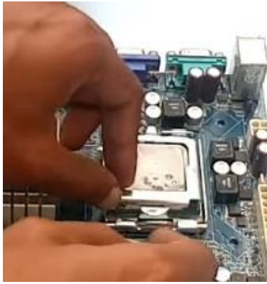
Figure 4. Close the CPU socket. From How to Make or Assemble Desktop CPU Step by Step At Home | How to Build a Computer with used Parts . ( https://www.youtube.com/watch?v=m_-G9Cacx2U , accessed 11/12/2020)
