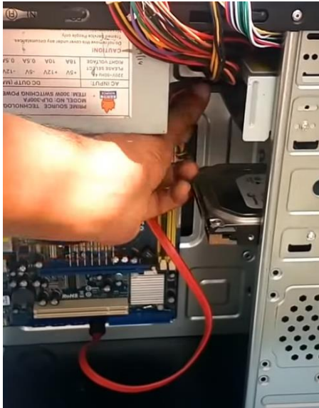
Figure 25. Connect SATA cable to motherboard and CD ROM. From How to Make or Assemble Desktop CPU Step by Step At Home | How to Build a Computer with used Parts .
