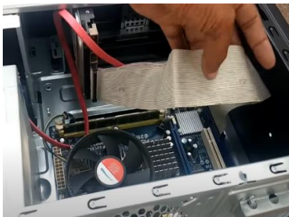
Figure 26. Connect IDE cable to IDE slots of motherboard and hard disk. From How to Make or Assemble Desktop CPU Step by Step At Home | How to Build a Computer with used Parts .
