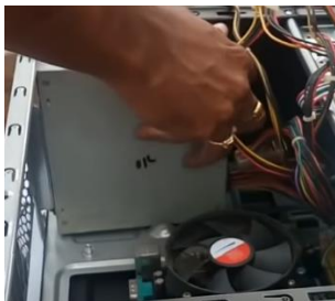
Figure 11. Mount power supply into case. From How to Make or Assemble Desktop CPU Step by Step At Home | How to Build a Computer with used Parts . ( https://www.youtube.com/watch?v=m-G9Cacx2U , accessed 11/12/2020)
