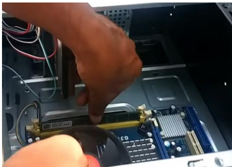
Figure 21. Unlock the slot on motherboard and insert RAM into the slot. From How to Make or Assemble Desktop CPU Step by Step At Home | How to Build a Computer with used Parts . ( https://www.youtube.com/watch?v=m-G9Cacx2U , accessed 11/12/2020)
