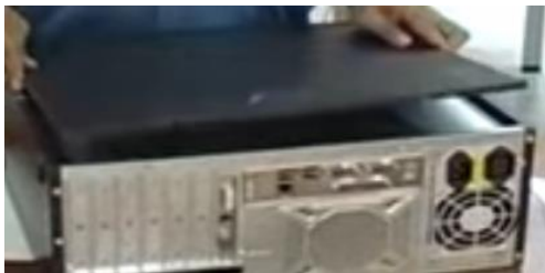
Figure 29. Place the side cover back on. From Asas Pemasangan Sistem Komputer (ESS207) ( https://www.youtube.com/watch?v=ctK58A71DTs , accessed 11/12/2020)
