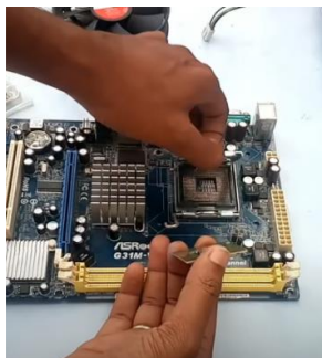
Figure 2. Open the CPU socket. From How to Make or Assemble Desktop CPU Step by Step At Home | How to Build a Computer with used Parts . ( https://www.youtube.com/watch?v=m_-G9Cacx2U , accessed 11/12/2020)
