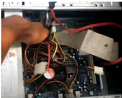
Figure 27. Connect power cable to motherboard, hard disk, graphic cards and accessories. From How to Make or Assemble Desktop CPU Step by Step At Home | How to Build a Computer with used Parts .
