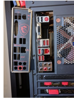
Fig 6. An IO shield next to the ports
