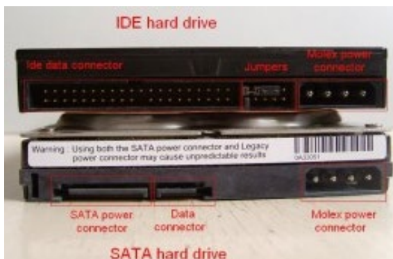
Fig 20. The different types of interfaces of a hard drive
