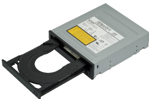
Fig 17. An optical disc drive can allow use of discs such as DVDs, CDs and Blu-ray.
