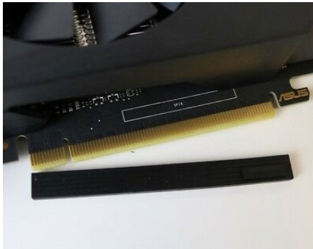
Figure 24. Example of a graphics card's pin cover
