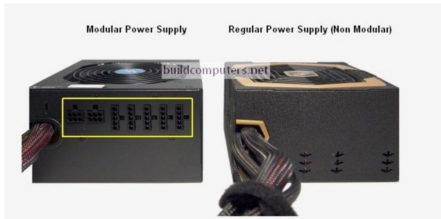
Fig 9. A modular and a non-modular power supply unit. Notice that the modular power supply has extra ports while the non-modular one has more wires running through it.
