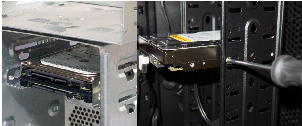
Fig 19. Example of how to install a disk drive
