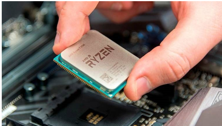
Fig 2. Example of how to properly hold a processor
