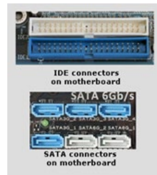
Fig 21. The connector ports on a motherboard
