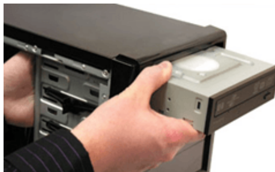
Fig 18. Example of how to install an optical drive.
