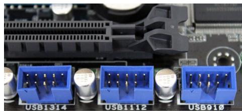
Fig 16. Example of USB Headers
