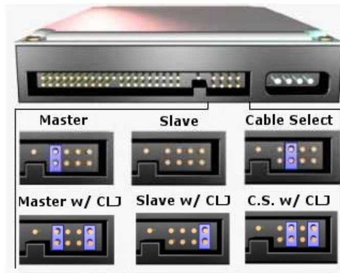
Figure 22. A jumper setting diagram for a hard drive
