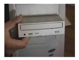
• Slide in the CD ROM drive into the computer case and make sure you install it right side up so that you can insert a disk.
