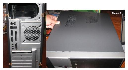
• Place the side cover back on and secure the side panels with case screws.
