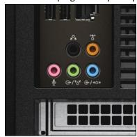
• Connect speakers and microphone into 2.5 mm sockets.
