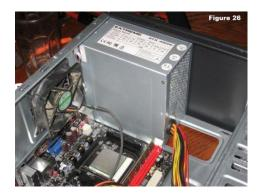
• Put the power supply to its place and screw it into place with four screws. Tighten it.
