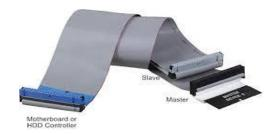
IDE cables are used to connect hard drives and optical drives to each other and to the motherboard in parallel connection. The two most common types of IDE ribbon cables are the 34-pin cable used for floppy drives and the 40-pin cable for hard drives and optical drives.
