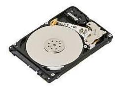
A hard disk is an electro-mechanical data storage device that stores and retrieves digital data using magnetic storage. There are two types of hard disks which are internal hard disk and external hard disk. Example models of hard disk are SATA hard disk and IDE hard disk.
