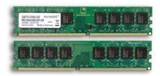
RAM (Random-access memory) is a volatile memory that store current running program. It is used to store working data and machine code. There are two main types of RAM which are
