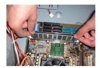
Press to open the clips at both ends of the RAM mounting slot. Line up the notch of the RAM stick with the mounting slot. Sit down the RAM and press it tightly into the slot. The tabs
