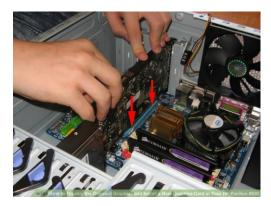
Remove the card gently from its bag, making sure that the card does not touch any electric component. Insert it straight into the empty PCI-e slot and apply even pressure to the top until it is placed correctly. Then, use case screws to secure the graphics card to the chassis.
