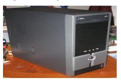
Install the side panels and make sure all the screws are tight enough to hold the side panels. This give a good protection from physical damage to the hardware inside. The computer is now ready for the software installation.
