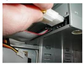
First, Insert the CD-ROM drive inside the drive bay slowly to make sure it will not get stuck. Then, fasten the CD-ROM drive with the locking mechanism and connect the SATA power cable to the CD-ROM drive. Connect the other end of the SATA power cable to the power supply and then Connect the SATA data cable to the CD-ROM drive. Lastly, connect the other end of the SATA data cable to the motherboard.
