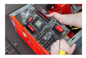
First, find the standoffs and install the standoffs as the standoffs is the place to put the motherboard. Then, place motherboard on the standoffs where the holes and the standoffs should line up. If the motherboard does not come out of the case, gently force the motherboard to fit in the panel. Secure the board with screws.
