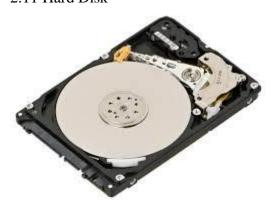
Generally, users can set the hard disk jumper to Master or Slave. Hard disk can store digital data by using magnetic storage. Example models of hard disk are Seagate BarraCuda, Toshiba X300 and WD VelociRaptor.
