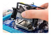
If possible, spread thermal paste to the back of the CPU. Seat the heatsink/cooler of the CPU and set it in place. Make sure the heatsink/cooler of the CPU has been clipped tightly. Attach the power cable to the cooler fan to the motherboard connector.
