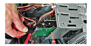
Connect the IDE cable, SATA cable and install the power supply. Connect the SATA power to a storage drive. Make the wire neat by tied it. This will help it in saving the space and hardware cooling.
