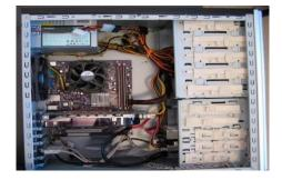
Connect the switch wire and USB onto the motherboard correctly. Note that every device that has been installed needs power. The power supply connectors are shown. The motherboard has two power connections, and there are two connectors specifically for SATA devices. The other
