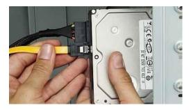
First, fit the hard disk into the bay. Then, plug in the SATA power cable. Be extremely careful when plugging it in, because any downward pressure can break the clip surrounding the power connector. Then, connect the SATA cable into the rear of the hard disk. Lastly, plug in the SATA cable into the motherboard.
