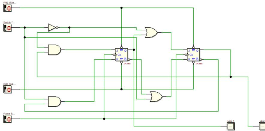
3. Investigate the behavior of the counter by observing the next state of the counter for all combination of Present State and X values. Complete the Next State table of the counter in Table 2. Ensure the Switch 0 is in HIGH state.
