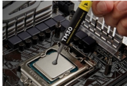
Picture 6: Applying thermal paste to the processor
