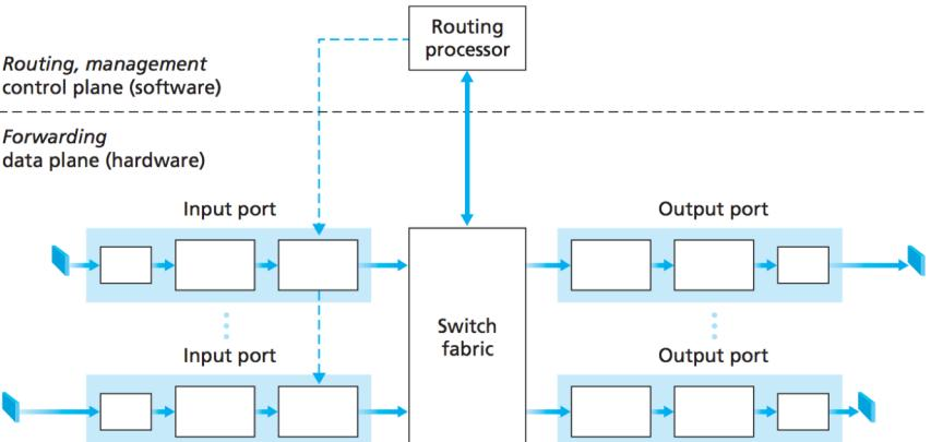
**Figure:** A high-level view of a generic router architecture
