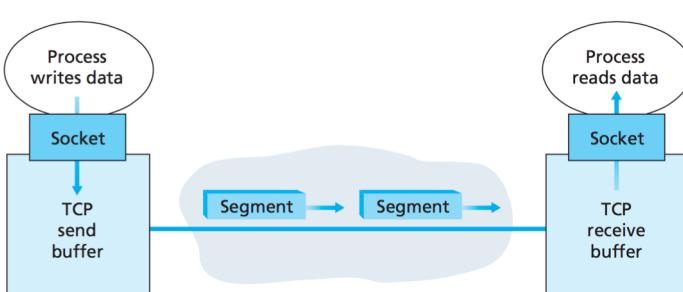
**Figure:** TCP send and receive buffers
