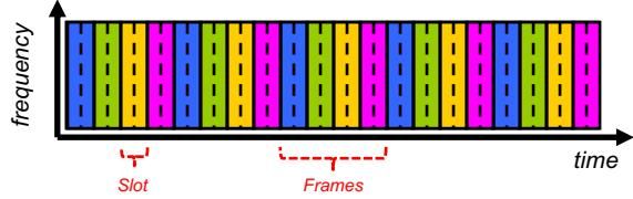
Users will access media (e.g. cable) based on different **time slot (second)** allocation
