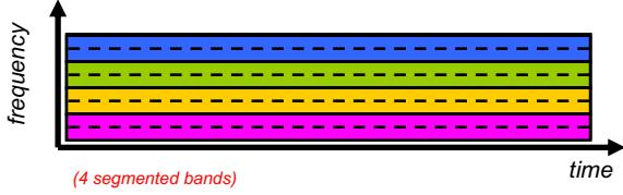
Users will access media (e.g. cable) based on different **frequency (Hz)** allocation
