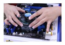
Then, install the heat sink neatly on the processor.
