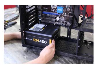
The power supply is placed under the motherboard and sits against the back of the case. After placing well, the power supply can be screwed tight.
