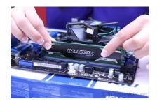
Place each RAM stick in a slot and force it down on both sides equally before the clips interact.
