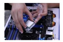
To show the socket and its pins, remove the CPU retention bracket lever. These are extremely sensitive and simple to bend, so when working around the socket carefully.
