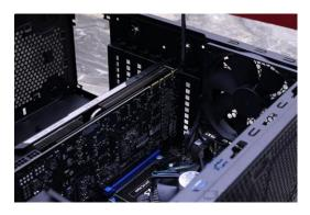
Screw the graphics card tightly with the holes originally provided from the graphics card which have the same diameter holes as blanking plates.
