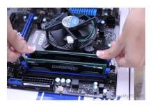
Ensure the tabs are locked into place by clipping down each side of RAM.
