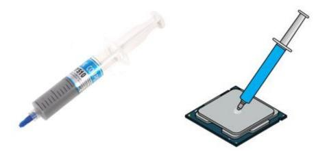
Thermal paste is a silvery-grey substance that is applied to the processor before installing a cooling solution. The function of this is to eliminate air gaps or spaces within the area. It is important as it could ensure the efficiency of heat transfer from processor to water block of CPU cooler.
