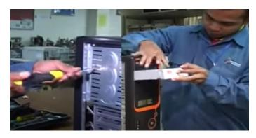
As all the CPU have the CD ROM, the CD ROM will be inserted once after the installation of the graphics card because the graphics card is placed in a deeper position compared to CD ROM. For this task, we need at least two people, one of the persons holding the CD ROM and the other one will be in charge of screwing it.
