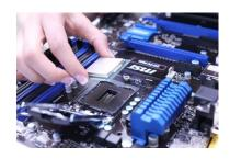
On the CPU socket, locate the corresponding marking and insert the CPU so that the markings are lined up.
