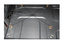
Place in the rear of the case the I/O bezel plate into the opening and instal standoffs in the case. The standoffs screw into the mounting holes of the motherboard. For correct positioning, check the screw hole positions on the motherboard.
