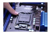
By pressing down and out of the processor socket, raise the CPU retention bracket lever from under its latch. Bear in mind that this can differ slightly depending on the socket of your motherboard and it is best to refer to the manual that came with the motherboard.
