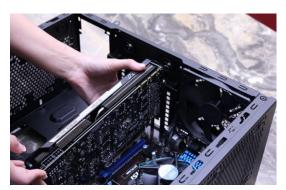
Lower the card into position and push down evenly at both ends until the clip engages.
