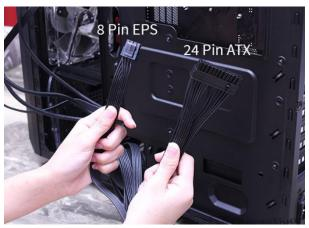
EPS power connector will be placed on top of the motherboard and the ATX is connected to the edge of the motherboard.
