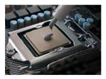
Apply a little bit of thermal paste on top of the CPU or processor. Make sure the chip is clean before doing this process.
