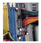
Connect the largest- cabling connector from power supply cabling to the motherboard power connector
