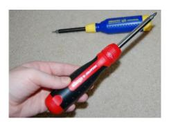
One of the most important and essential tools for the PC assembly. Computers are held together with screws and, luckily, nearly all types of screws used in computers are Phillipshead. The number-one most important tool for PC building is a Phillipshead screwdriver with a big bit, helpful to avoid stripping the head; a long shaft also aids in keeping the handle out of the way when working in tight spaces—it's a good idea to keep a short screwdriver around as well, for the same reason.
