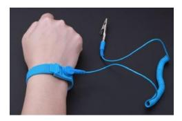
The ESD wrist strap is used to discharge static electricity on the body to ground. It is important to prevent static build up which could harm the electronic circuit when assembly the pc.
