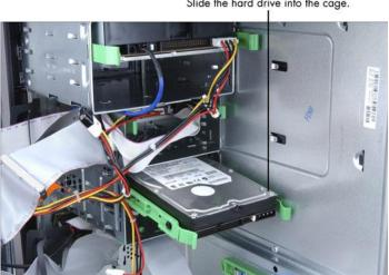
Slide the hard drive into the cage.
