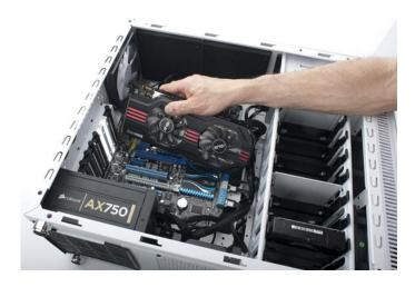
• Screw on the graphic card holder so that it is neat and not easily fall off.
