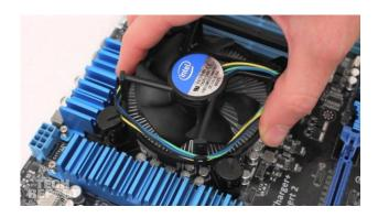
• Please make sure that the heat sink and fan have been clipped tightly.
