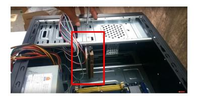
After that you start adding the screws to hold the device in place.
