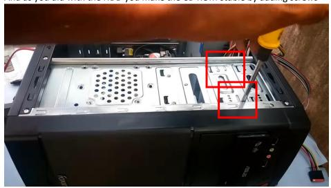
Then you connect the CD ROM. CD ROMs can be SATA or IDE for IDE you connect the cable to the motherboard using SMPS 12 pin connector or ATX 24 pin connector or ATX 4 pin connector.
