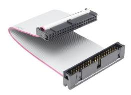
You connect one end to the HDD and the other to the motherboard. The end with pointy metals is called the male end and the other one is called the female end. The male end is attached to the HDD and the female end is attached to the motherboard.
