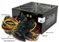
PSU or Power Supply Unit is the one of the most important component for building PC, without it we can't turn on our PC. It procedure is to convert AC power to low-voltage DC power in order the other components of a PC would be working properly. There are three types of PSU: AT, ATX, and ATX-2. Most used nowadays is ATX-2.
