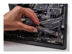
After installing the SSD there is a hole in the back of the SSD and there is a hole in the motherboard to add a screw so that the SSD become stable and don't move or get out of the socket.
