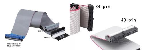
IDE cables used to connect some hard drives and optical drives to each other and to the motherboard. The two most used types of IDE ribbon cables are the 34-pin cable used for floppy drives and the 40-pin cable for hard drives and optical drives.
