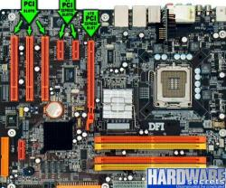
PCie slots are slots commonly exist at motherboard, that comes in different sizes x1, x4, x8, x16 and different generations as well. The number after the x mean how many lanes (data travels to and from the PCIe card) that PCIe slot has. A PCIe x1 slot has one lane and can move data at one bit per
