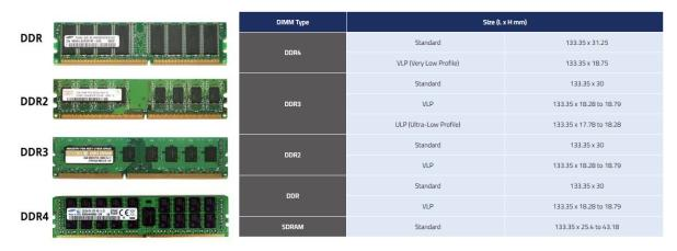
Random Accessible Memory or RAM is an essential part of a computer's hardware because it stores data for programs when they are processed by the CPU. The data only stored temporary (short term), so when we turned off the PC, data which stored in RAM will be closed. And there are several types of RAM: SRAM (Static random-access memory), SDRAM (Synchronous DRAM), and DDR SDRAM, which DDR refers to double data rate. And DDR comes with 4 models, DDR only until DDR4.
