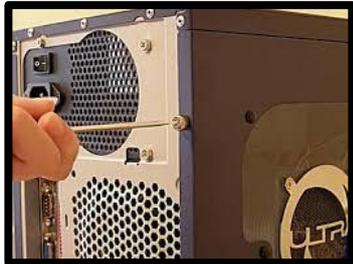
Place the side cover back on and secure the side panels with case screws.
