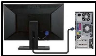
Finally connect the CPU with monitor by plugging into display ports
