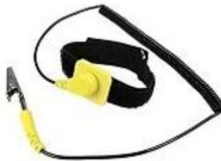
An anti-static wrist strap (or band) is a bracelet-type device you wear on your wrist which connects to an electric socket, and if any electrical charge builds up between you and your hardware components, the charge is safely dissipated through to the socket (avoiding a spark and potentially causing damage to your parts). The importance of this tool is an easy way to discharge any electrical build up compared to using the gloves.
