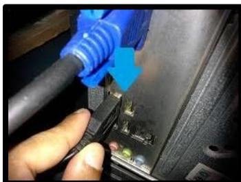
Connect peripheral devices which include keyboard, mouse, wireless network dongle, printer and webcams with your CPU by plugging into USB port.
