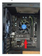
Then remove the case expansion bracket after that, mount the Graphic card to the PCIe slot.
