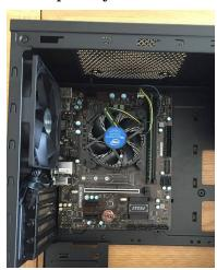
Next Put screw and tighten them (don't screw TOO tight it may damage the motherboard)
