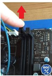
Next insert the RAM by giving it a firm little press from the top, but never use too much force because it shouldn't require a crazy amount of force if you're aligned it properly. To properly seat it all the way, it might be easier to press down on either side one at a time until the slots locked(the slot will automatically locked the ram if inserting it in properway)
