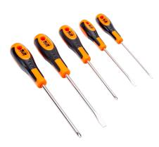
Screwdriver is used to screw or unscrew all the screw used to held together almost all of the component in a PC. There are several type of screwdrivers which is philips, flathead, hexhead. Screwdrivers is very important because almost all of the components in the PC are held together using screw.
