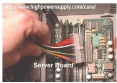
then the 8-pin connector to the CPU Slot
