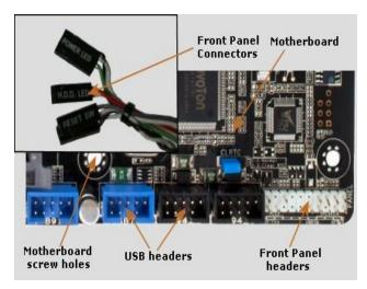
Then connect the cable to right headers on Motherboard
