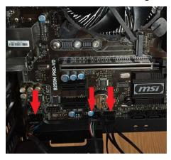
Step 10 - Connecting the Component cable to PSU first Connect the 24-pin connector to the motherboard
