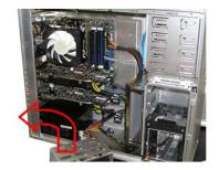
Next screw openings on the rear of the case with the PSU, and keeping in mind that holding the PSU solidly set up feel free to fasten them with the screws that ought to have been furnished with your PSU. Something else, use screws gave by the case. Fix them pleasant and solidly, yet not excessively close.
