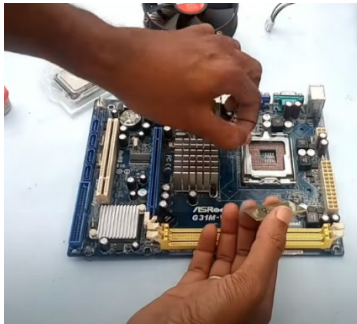
Figure 1. Lift metal rod of socket. From How to Make or Assemble Desktop CPU Step by Step At Home | How to Build a Computer with used Parts. ( https://www.youtube.com/watch?v=m_-G9Cacx2U , accessed 11/12/2020)
