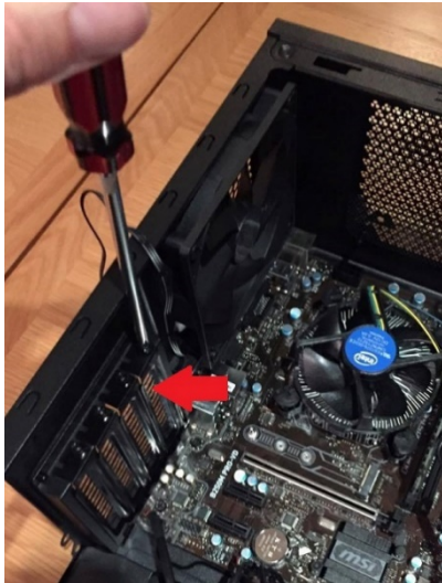
Figure 16. Unscrew bracket next to PCIe slot. From How to install a graphics card . ( https://www.build-gaming-computers.com/how-to-install-graphics-card.html , accessed 11/12/2020)
