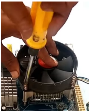
Figure 9. Tighten the screws on the heatsink and fan. From How to Make or Assemble Desktop CPU Step by Step At Home | How to Build a Computer with used Parts .
