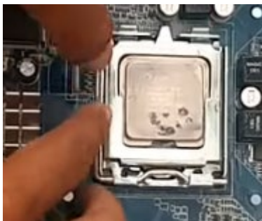
Figure 5. Lower the metal rod next to the socket. From How to Make or Assemble Desktop CPU Step by Step At Home | How to Build a Computer with used Parts . ( https://www.youtube.com/watch?v=m_-G9Cacx2U , accessed 11/12/2020)
