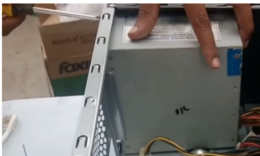
Figure 12. Secure power supply to case with screws. From How to Make or Assemble Desktop CPU Step by Step At Home | How to Build a Computer with used Parts . ( https://www.youtube.com/watch?v=m-G9Cacx2U , accessed 11/12/2020)
