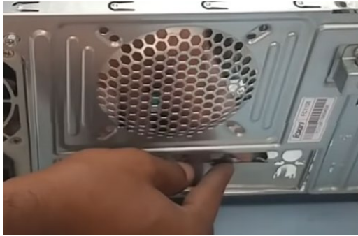
Figure 13. Install Input Output Shield into case. From How to Make or Assemble Desktop CPU Step by Step At Home | How to Build a Computer with used Parts . ( https://www.youtube.com/watch?v=m-G9Cacx2U , accessed 11/12/2020)
