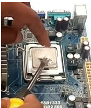
Figure 6. Apply thermal paste. From How to Make or Assemble Desktop CPU Step by Step At Home | How to Build a Computer with used Parts . ( https://www.youtube.com/watch?v=m_-G9Cacx2U , accessed 11/12/2020)
