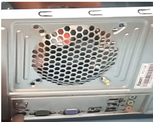
Figure 14. Adjust motherboard to the Input Output Shield. From How to Make or Assemble Desktop CPU Step by Step At Home | How to Build a Computer with used Parts . ( https://www.youtube.com/watch?v=m-G9Cacx2U , accessed 11/12/2020)
