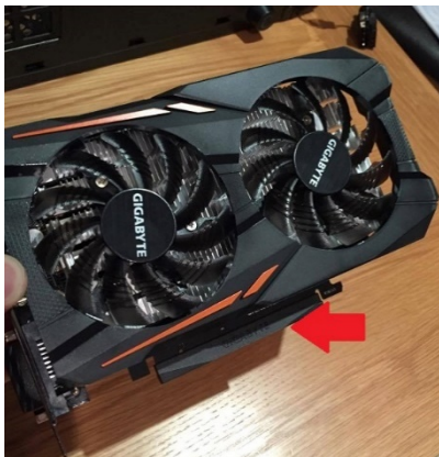
Figure 17. Unlock retention clip and remove cover of graphic card. From How to install a graphics card . ( https://www.build-gaming-computers.com/how-to-install-graphics-card.html , accessed 11/12/2020)
