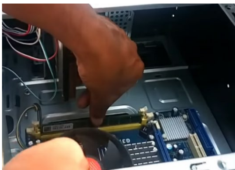
Figure 21. Unlock the slot on motherboard and insert RAM into the slot. From How to Make or Assemble Desktop CPU Step by Step At Home | How to Build a Computer with used Parts . ( https://www.youtube.com/watch?v=m-G9Cacx2U , accessed 11/12/2020)
