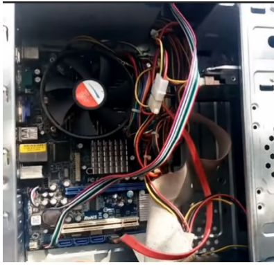
Figure 28. Connect USB cable and audio cable to motherboard headers. From How to Make or Assemble Desktop CPU Step by Step At Home | How to Build a Computer with used Parts . ( https://www.youtube.com/watch?v=m_-G9Cacx2U , accessed 11/12/2020)
