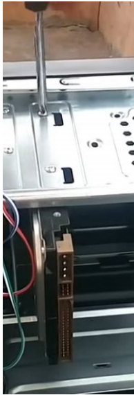
Figure 20. Secure hard disk with screws. From How to Make or Assemble Desktop CPU Step by Step At Home | How to Build a Computer with used Parts . ( https://www.youtube.com/watch?v=m-G9Cacx2U , accessed 11/12/2020)
