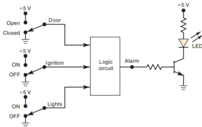
Figure above shows a diagram for an automobile alarm circuit used to detect certain undesirable conditions. The three switches are used to indicate the status of the door by the driver's seat, the ignition, and the headlights, respectively. Design the logic circuit with these three switches as inputs so that the alarm will be activated whenever either of the following conditions exists:
