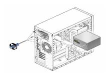
Tighten it by screwing each side of the power supply using a screwdriver.
