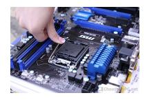
Finally, push down the CPU retention bracket lever to lock the processor in place.
