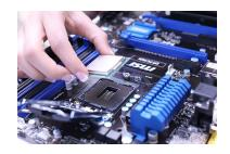
On the CPU socket, locate the corresponding marking and insert the CPU so that the markings are lined up.
