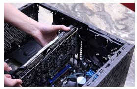
Lower the card into position and push down evenly at both ends until the clip engages.
