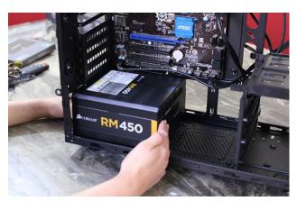
The power supply is placed under the motherboard and sits against the back of the case. After placing well, the power supply can be screwed tight.
