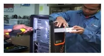
As all the CPU have the CD ROM, the CD ROM will be inserted once after the installation of the graphics card because the graphics card is placed in a deeper position compared to CD ROM. For this task, we need at least two people, one of the person holding the CD ROM and the other one will be incharge of screwing it.
