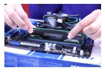
Place each RAM stick in a slot and force it down on both sides equally before the clips interact.
