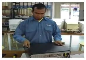
Lastly the case will be screwed to close the internal part of the CPU to prevent any further damage from the outside force and to avoid the accumulation of dust too.
