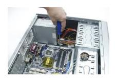
After aligning the motherboard to its place, use a screwdriver to tighten the screws.
