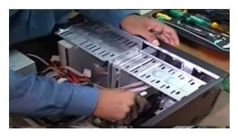
Hard- Disk is a must for every CPU. The CPU will be placed down by side so that it will be easier to place and screw the hard-disk driver inside the CPU.
