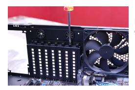
For the installation of graphics card, PCle blanking plates need to be removed to insert the graphics card in.
