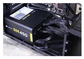
The power cabling is important for our CPU also as it connects directly to our motherboard and if we placed the cable wrongly, the motherboard might spoil 20/24 pin ATX power cable and the 4/8 pin EPS power cable will be connected to the motherboard but in a different position.
