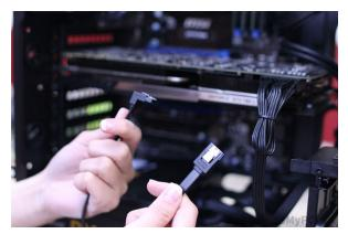
SATA cable actually have two connectors which is SATA data and SATA power and both connectors is in "L" shape
