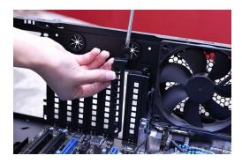
For graphics card, it is usually placed at the topmost PCle x16 and for the second PCle blanking plate is for the 2nd graphics card if using dual slot graphics card.
