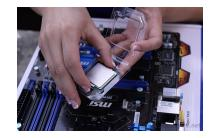
To show the socket and its pins, remove the CPU retention bracket lever. These are extremely sensitive and simple to bend, so when working around the socket carefully.
