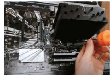
doing that we should apply thermal paste between the heat sink and CPU and this step is very important because it will help to keep the processor cooled without the need to clean the heat sink every week.
