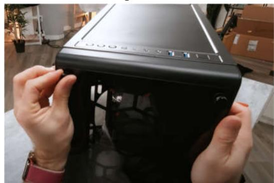
case correctly, after that we will put the front panel back in its place and make sure that all cables in the case are connected and working with the motherboard. Moving on after closing the case we will connect the PC with the screen using HDMI cable and connect the mouse and keyboard using USB ports to control the device. Now we can click the power button and be proud that we assembled a fully working PC.
