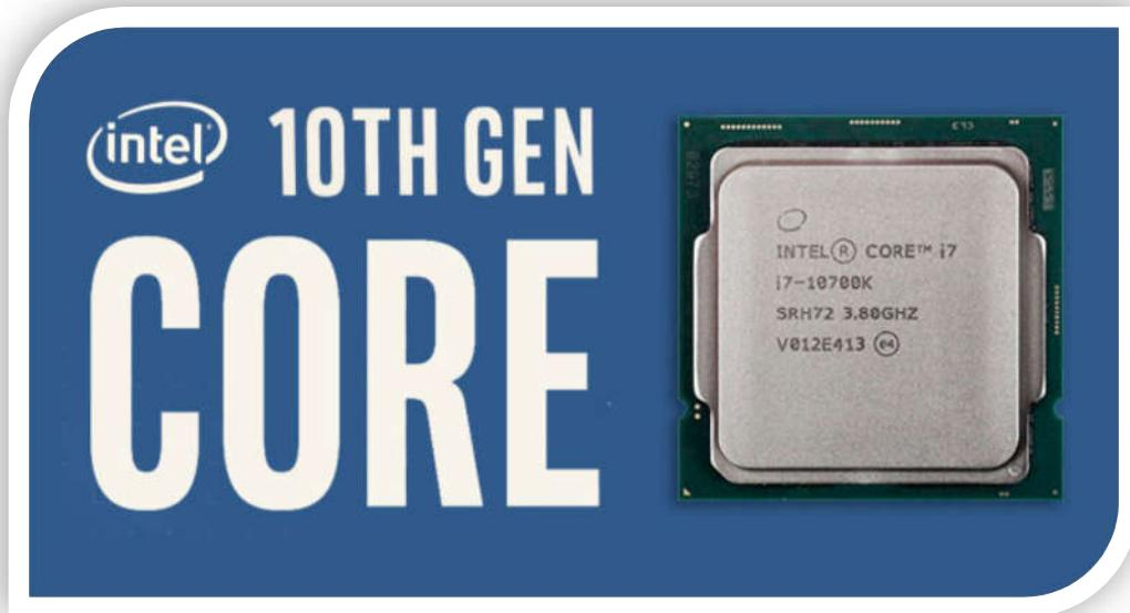
The CPU is the unit that performs most of the processing on a computer. To manage guidelines and statistics float to and from other parts of the computer, by performing the fundamental arithmetic, logic, controlling, and Input/output (I/O) operations, the principal components of CPU includes Arithmetic Logic Unit (ALU), Control Unit (CU), and Registers/The Memory Unit (MU). Intel 10th gen core i7 is a clear example of processors used in PCs recently due to its performance and cost.
