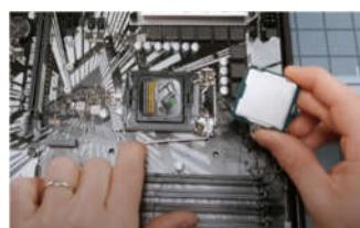
Moving to installing the CPU we can go ahead and install it, step one is to push down the lever pull it out and then the retention plate should move out of your way then we're going to see this little golden triangle here we're going to line that up with the dot at the corner of the socket on.
