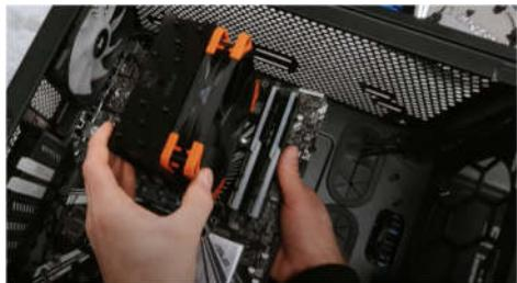
Lastly, after a long journey of assembling the PC, we now reached the best moment for anyone who is putting the last touches to construct the fully working system. We need to ensure that the motherboard and all components included in it fitted in the
