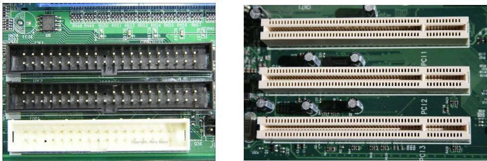
IDE slots are used to connect hard drives and optical devices to the motherboard, While PCI slot is used to attach and connect devices to the motherboard such as modems, network cards, and sound cards. Usually, both slots are built-in with the motherboard as a port, IDE 40 pin and PCI-E 1.0 are very known as the most used slots.
