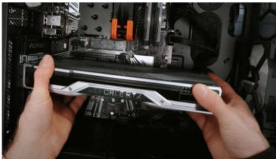
Installing GPU recently, is better to be the last component to install in the PC assembly process. GPU installation is plugged to motherboard by PCI cables from the card to the slot in motherboard easily as a tip we need to make sure
