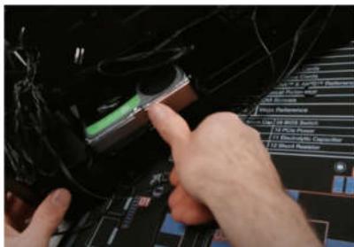
Actually, Hard drives are the easiest part to install nowadays all we need to do is to slide the hard drive in its place in the case then we can use the SATA cable or other cable that can work with the HDD and plug one end into the
