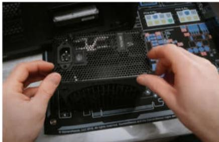
To install the power supply, we can keep it outside the case or keep it inside the case if there is a space available. We will use the screws that usually came in the same box of it to secure it inside the case as we recommend, lastly, we need to connect it by AC adapter to the motherboard.
