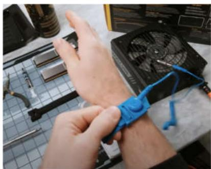
The first thing we're going to do is get ourselves static-safe so we're going to use the anti-static equipment in order to dissipate any static that's built up on our bodies. We just need to put the alligator clamp on a metal part and the other end either on your wrist or as preferred on your ankle this way is great because it will not be on your way while you're trying to build the PC.
