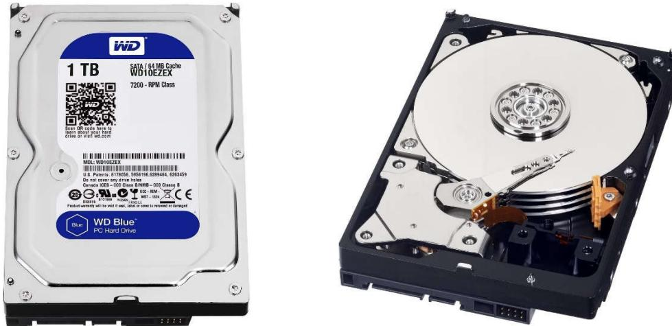
is an electromechanical data device that stores and retrieves digital data using a data-storage medium and one or a lot of rigid quickly rotating platters coated with magnetic material. HDDs are a kind of computer memory, retentive keep data even once battery-powered off. As an example, Western Digital 1 TB WD10EZEX is very good that performs very well and at a low cost.
