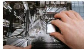
recommend to shake it slightly to be placed firmly. Next, we're going to drop the plate down making sure that it stays clear of hitting the screws, and lower the arm pull it out and put it under the retention mechanism.
