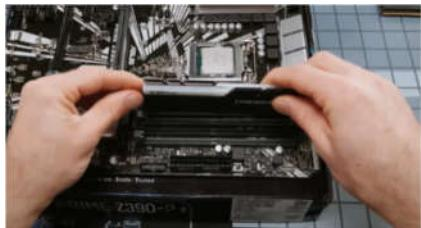
We can Install RAM by lining up the memory with the slot, make sure you carefully check the position of the notch so you can see in the image. Then, pull back the tabs remember to do that slowly to not break the slot, push firmly from both sides until you hear a click on each end, and that's all.
