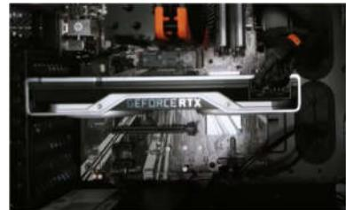
that all pins is straight and not bended before installing it. We also need to apply an even pressure while placing GPU in its place securely and firmly, in the other hand we need to line up the I/O while installing the card I the case.
