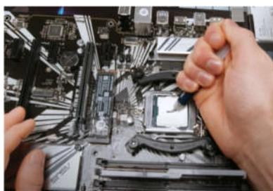
In this step we will plug the heat sink on the CPU to ensure that our processor is cooled probably well, first thing we need to do is to align the heat sink with the screws at the motherboard to secure it in its place but before
