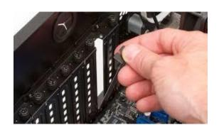
**6.1** Remove the expansion slot cover from the rear of the computer case.
