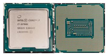
Central Processing Unit, CPU is the brain of computer. Just like its' nickname, CPU processes and executes instructions so that the computer works. It receives input, processes the input, stores the data and produces output.
