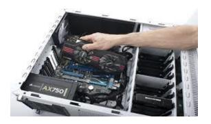
**6.2** Slot the graphic card into PCI expansion slot on the lower half of the motherboard. Line it up and press down firmly to seat the card.
