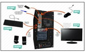
**10.2** Connect peripheral devices which include keyboard, mouse, wireless network dongle, printer and webcams with your CPU by plugging into USB port.
