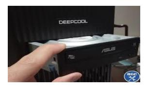
**8.2** Mount in the CD ROM drive in the case by fixing it with screws.
