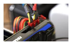
**6.4** Plug in the power connector from power supply into graphic cards connector. (if existing – not all graphic cards require external power)
