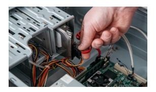
**7.2** (a) If you are installing SATA hard disk drive, connect the hard disk drive using SATA cable to SATA slot on the motherboard.
