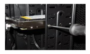
**7.1** Mount the hard disk drive in the case drive bays. Fix the drive in place with screws.
