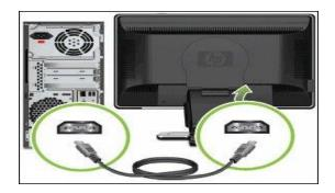
**10.4** Finally, connect the CPU to monitor by plugging into display ports.
