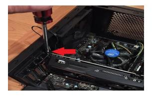
**6.3** Put in the screw to hold the graphic card.
