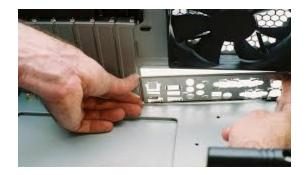
**5.2** Install the motherboard I/O plate.
