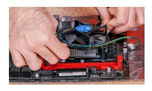
**2.2** Install the CPU heatsink/cooler with fix in position.
