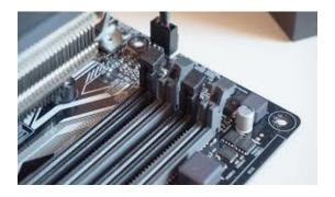
**3.1** Press to open the clips at both ends of the RAM mounting slots.
