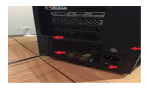
**4.2** Fasten the screws to the case mounting point.
