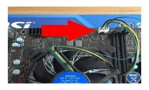
**2.3** Plug the power cable attached to the cooler fan into the motherboard connector.
