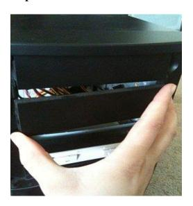
**8.1** Remove the front panel from the computer case where the CD ROM drive will sit.
