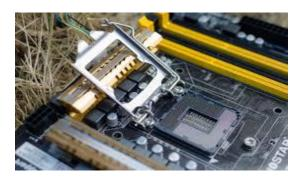
**1.1** Firstly, release the tension lever on the CPU.
