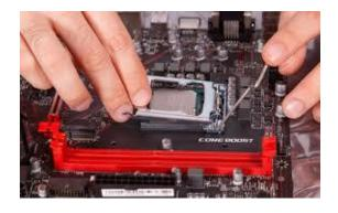
**1.3** Once the CPU settled correctly in the socket, press the tension lever back down.
