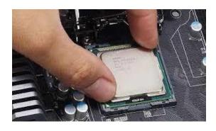
**1.2** Then, attach the CPU into the CPU socket.
