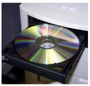
CD ROM is a short form for 'Compact Disc Read-Only Memory'. It contains data, which only can be played and can't be rewrite nor edited. CD ROM can be read by using a CD ROM drive which read the CD ROM by using laser light or electromagnetic waves.
