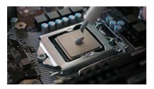
**2.1** Apply the thermal paste on the CPU.
