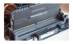
**3.3** Seat the RAM and press it firmly down into the slot. The tabs should automatically latch closed as you press the RAM down, securing the RAM in place.
