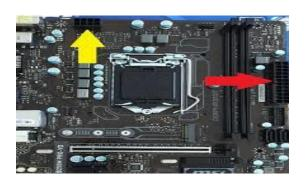
**4.3** Plug the largest cabling connector and 8-pin cabling connector from the power supply cabling into motherboard power connector and CPU power connector respectively.
