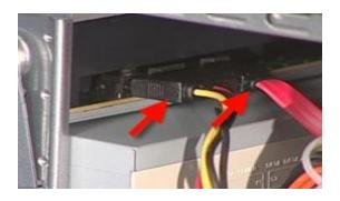
**8.3** Connect the CD ROM drive to the IDE slot or SATA slot on motherboard by using IDE cable or SATA cable. Connect power cables from the power supply to the CD ROM drive.
