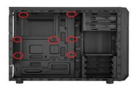
**5.1** Screw the motherboard standoff into the computer case.
