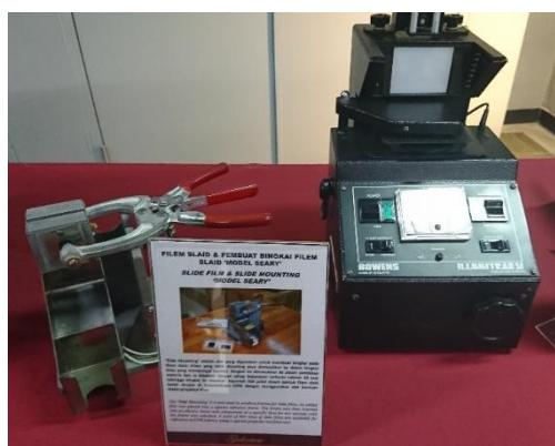
The 'Slide Mounting' is a tool used to produce frames for slide films. An edited film was placed into a special adhesive frame. The frame was then inserted into an electric brace and compressed at a specific heat for ten seconds until the frame was attached. A total of 600 titles of slide films are available for reference at UTM Library using a special projector machine tool.
