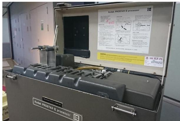
The 'Kodak Prostar II Processor' was used to cleanse the 16mm and 35mm sized microfilm of 'Recordak Micro-File' machine and the 'Zeutschel' microfilm camera machine. It also produced negative microfilms for UTM these. It was capable of processing microfilms with a speed of up to 10 feet per minute.
