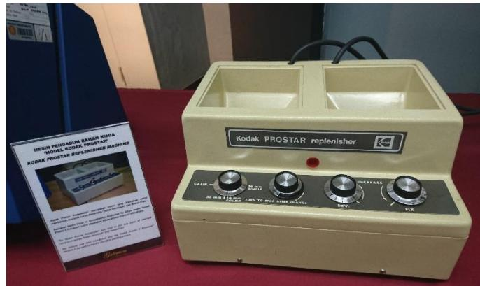
The 'Kodak Prostar Replenisher' was used to mix two types of chemical compound namely 'Kodak Developer' and 'Kodak Fixer'. The mixture was then transferred into the 'Kodak Prostar II Processor' machine to be used during the microfilm washing process.
