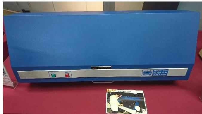
The ‘Silver Film Duplicator’ was used to produce negative to positive microfilm copies. The microfilm negative copies served as references to users while the positive copies were stored in UTM in Library special collection. The reasons for this was to ensure that the master copy of each UTM thesis is preserved and traceable in UTM Library collection.
