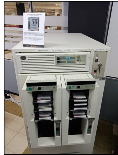
Figure 4: Magnetic tape unit with square shape tape.
