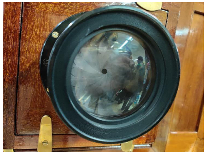
It had variable aperture which was adjusted using small metal fins inside the lens housing
