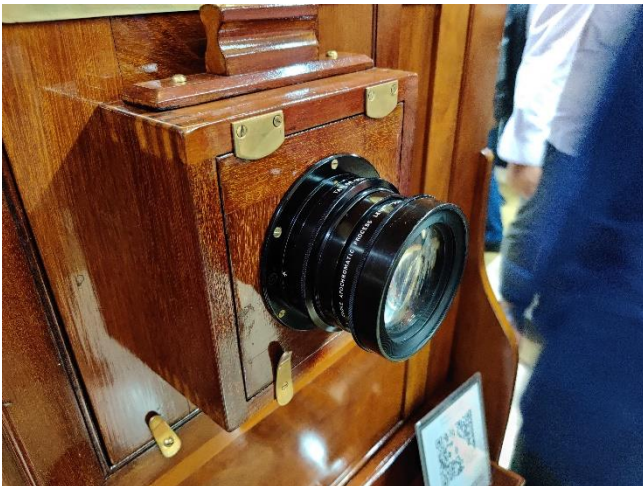
Hunter Penrose process cameras were huge in size coming in at 120cm long, 48cm depth, and 77cm height.
