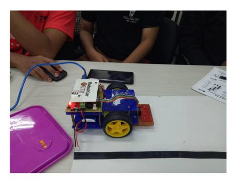
This is the coding for our ROBOKAR. At first we thought the coding would be complicated as we have studied things that is beyond our level. However, the coding is pretty simple, the Robokar have three sensors each detects a route, all we do is code when and how fast for the Robokar to move. For instance, in the code says if sensor detect number '2' it goes straight which basically the code is simple as that.
