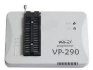
It is a device that can connect GAL 22V10 PLD directly into a program so that coded program can be loaded into the PLD to be tested on the ETS-5000 Digital Training kit.
