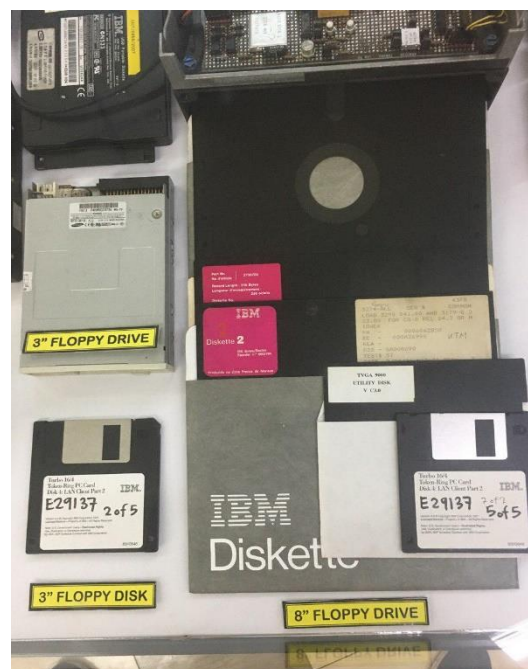
Figure 8.0 – 3" Floppy drive,3" floppy disk and 8" floppy drive
