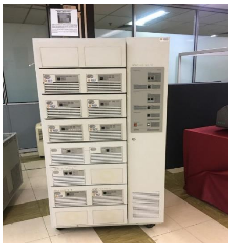
Figure 4.0 – Mainframe data storage, Model : IBM(9345B22)
