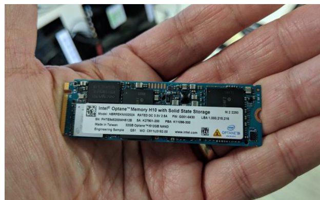
Figure 6.0 – Solid-state Drive that usually used in laptop
