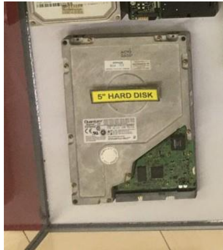
Figure 5.0 – Hard Disk Drive for CPU tower
