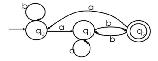
Construct the transition table of M. Which of the strings baba, baab, abab dan abaab are accepted by M?
