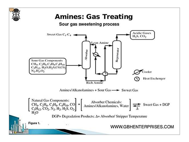
Amine gas treating, also known as gas sweetening and acid gas removal, refers to a group of processes that use aqueous solutions of various alkylamines which commonly referred to simply as amines, to remove hydrogen sulfide (H2S) and also carbon dioxide (CO2) from gases.
