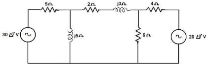
10.i) For the circuit shown, determine the current in (2+j3) ohm by using superposition theorem. (8)
