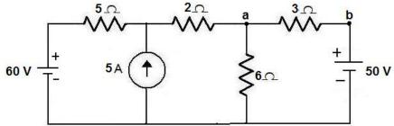
8. Determine the mesh currents  $I_1$  and  $I_2$  for the given circuit shown below (16)
