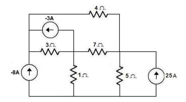
11.i) Using the node voltage analysis, find all the node voltages and currents in 1/3 ohm and 1/5 ohm resistances of figure. (8)
