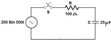
10. In the circuit shown in figure, the switch is closed at time t=0. Obtain i(t). Assume zero current through inductor L and zero charge across C before closing the switch.
