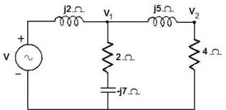
13. Using Mesh analysis, find current through 4 ohm resistor. (16)
