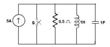
9. In the circuit shown in figure, find the current i. Assume that initial charge across the capacitor is zero. (16)
