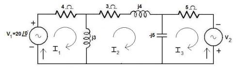
ii) Find the current through branch a-b using mesh analysis shown in figure below. (8)
