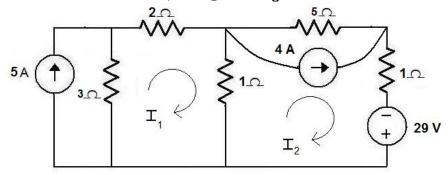
9. Find the node voltages  $V_1$  and  $V_2$  and also the current supplied by the source for the circuit shown below. (16)
