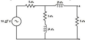
ii) Find the current in each resistor using superposition principle of figure. (8)
