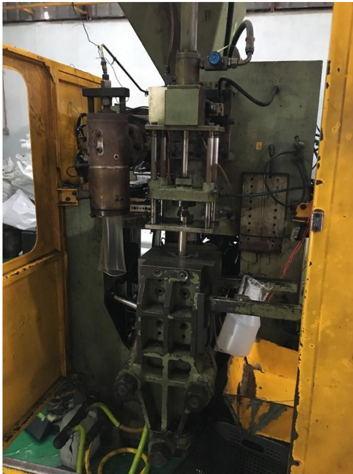
Figure 4.8: Extrusion blow molding machine at company
