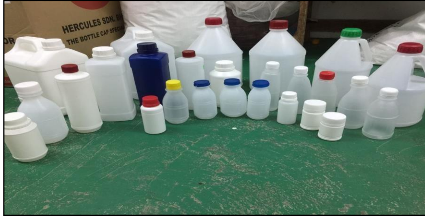
Figure 4.10: example product that been produced by extrusion blow molding machine
