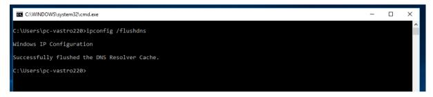
Figure C.5: ipconfig/flushdns result
