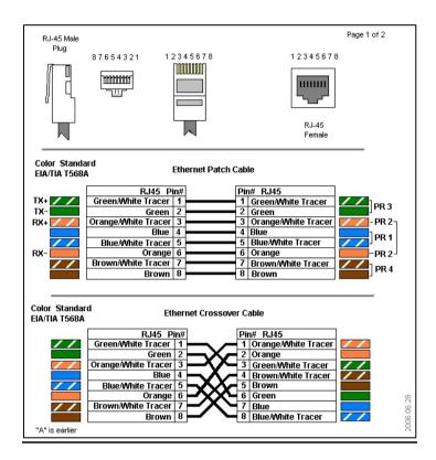
There are two things, RJ 45 Male plug, and RJ 45 female port. The colours of the wires are green, green with white tracer, orange, orange with white tracer, blue, blue with white trace, brown and brown with white tracer.
