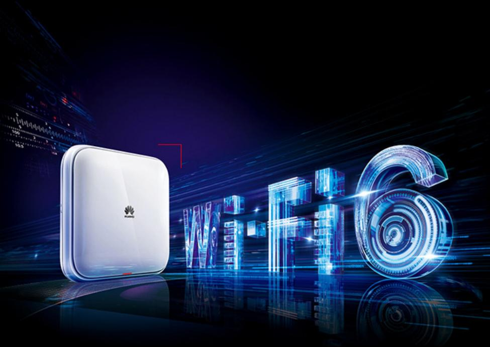
This device is very helpful for multi user scenarios for example in a company or in dorms. This device uses a lot of technologies that help spread the Wi-Fi signal such as MU-MIMO, BSS Coloring and OFDMA. These technologies spread the Wi-Fi in a smart way so that the places with more devices get a bigger bandwidth and Anti-interference/low latency. Also Multiple APs share spectrum resources which improve the spectral efficiency.
