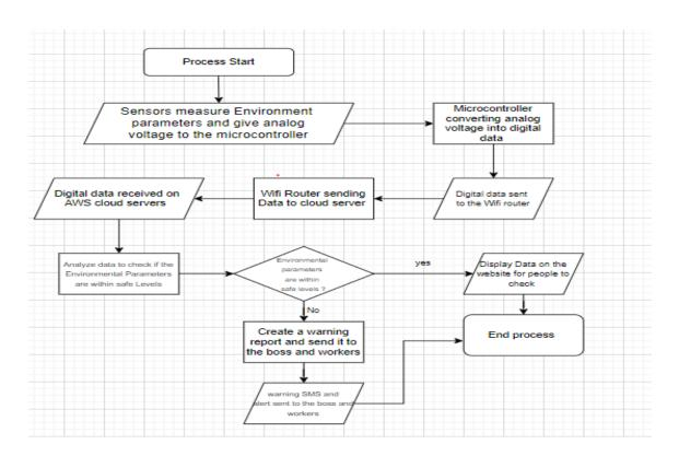
The flowchart diagram above shows how a smart weather reporting system works from getting the data from the sensors until the end of the process.
