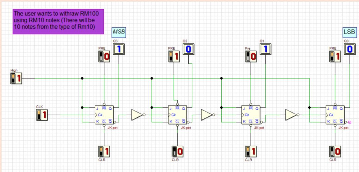
For visualized example, here the user wants to withdraw 100 ringgits using 10s, which will be 10 notes and this counter circuit's output is 1010 which corresponds to the value of 10 notes. Hence, the counter gives the count of exact number of notes.
