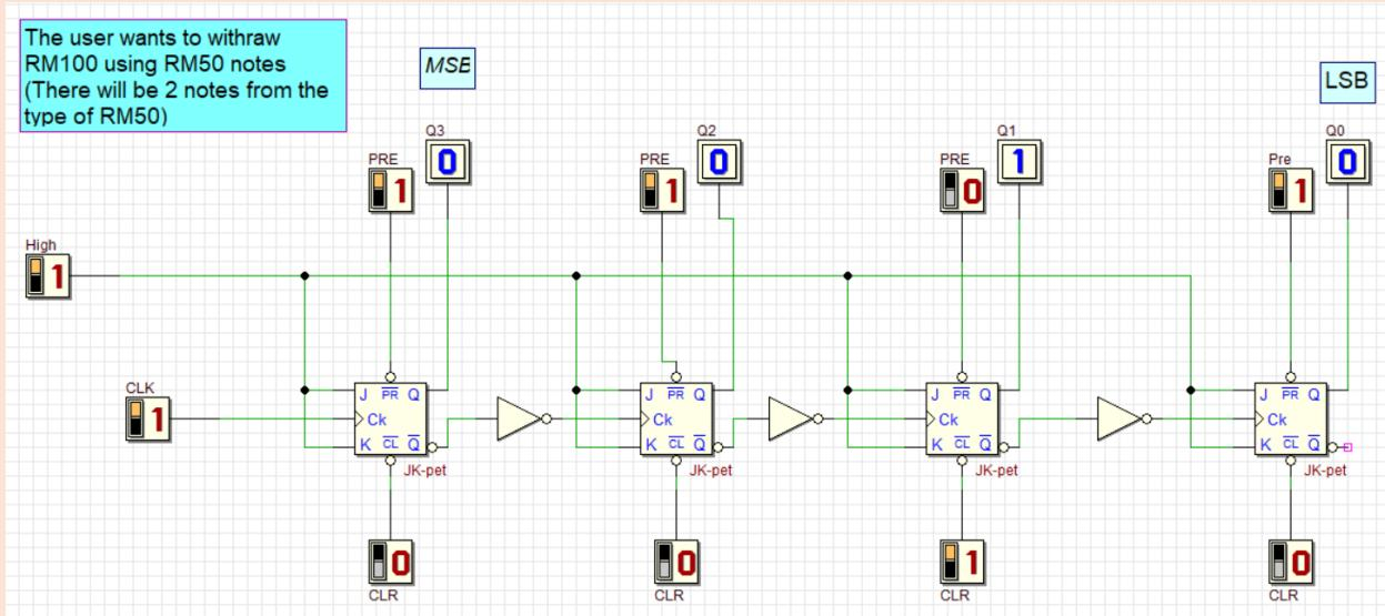
Again, by changing configuration of preset and clear of the same raw circuit, we can get the exact number of notes needed for the user to withdraw 100 ringgits using 50s. The output is 0010 (binary) which corresponds to the values of 2; the number of notes.
