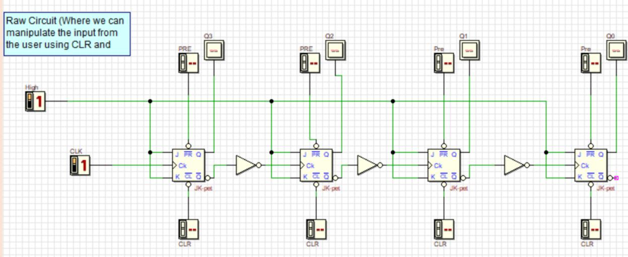
This is the sequential circuit used for manipulating the input from the users by making a counter based on JK flip flops. The most significant bit is Q3, and the least significant bit is Q0.
