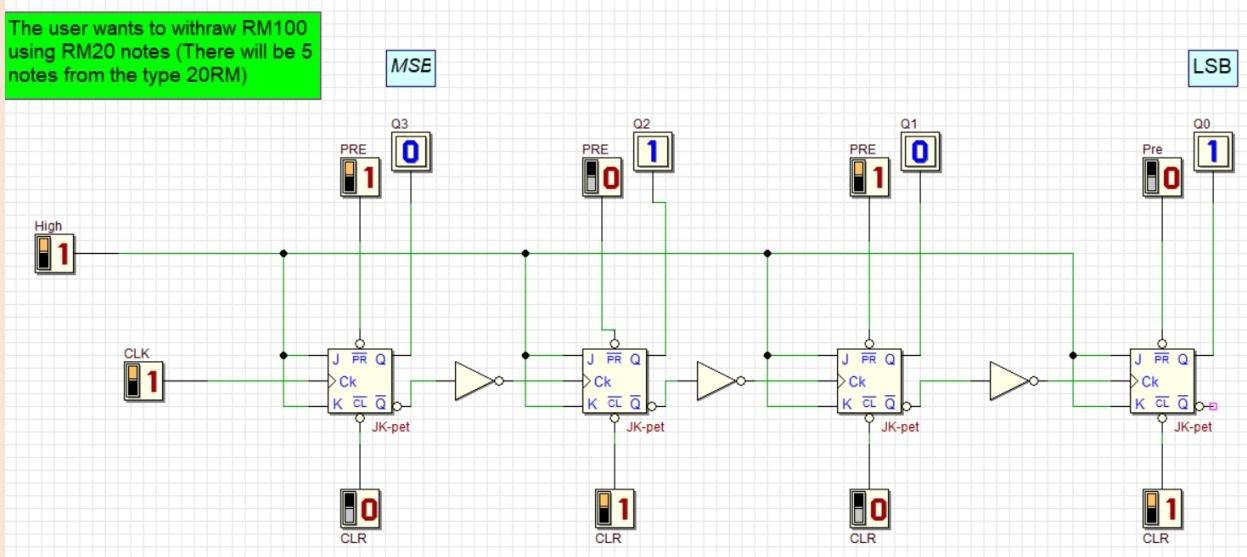
Changing configuration using preset and clear function, this circuit now shows the output of 0101(binary) which is 5 notes as needed by the user to withdraw 100 ringgits using 20s.
