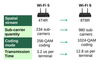
Wi-Fi 6 supports better multi-user experience which improved the multi-user experience by reducing terminal power consumption by 30% and enhancing gateway positioning as the control centre of smart homes.
