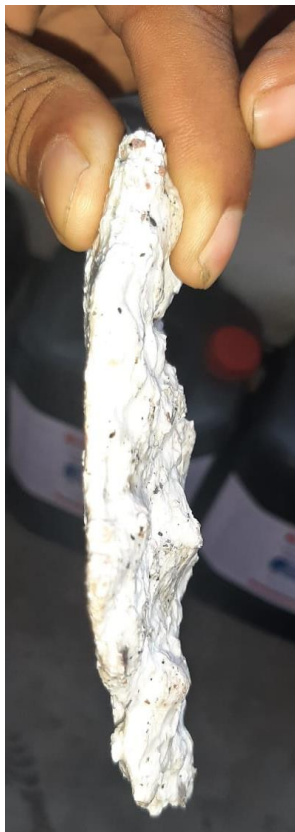
Figure 4.2.5.7 Scale of Water Tubing Section
