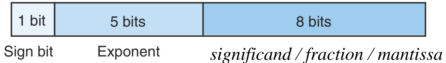
Figure: Example of 14-bit model for floating-point format.
