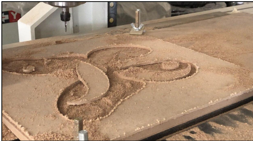
Figure 45 : Machining process of butterfly from ne machine
