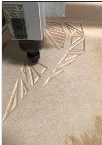
Figure 29 : Machining process of grill panel
