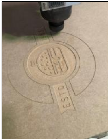
Figure 20 : Machining process of burger sign
