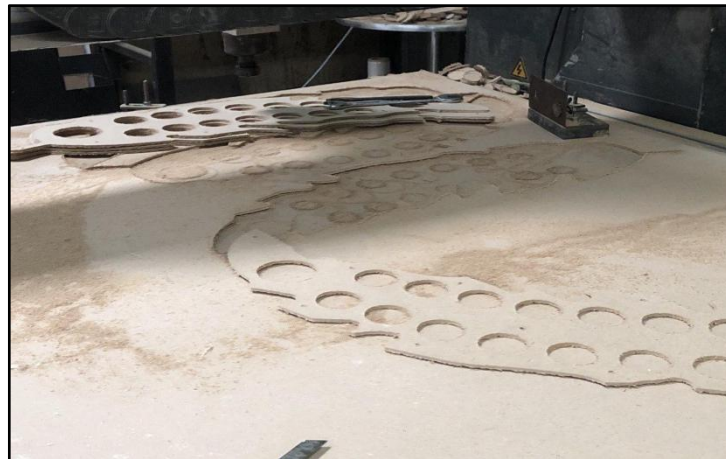
Figure 39 : Machining process of congkak
