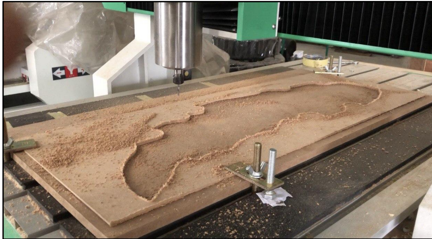
Figure 44 : Process of machining of congkak from new machine
