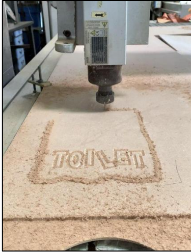
Figure 19 : Machining process of toilet sign
